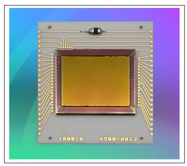
combined with the high quantum efficiency of the lattice matched InGaAs detector arrays enables impressive imaging in the SWIR and visible bands. Princeton Infrared Technologies, Inc. offers this low power array by itself on a ceramic submount or with a hermetic package. It is also incorporated in a set of camera electronics for a complete solution in our 1280SciCam or 1280MVCam.
